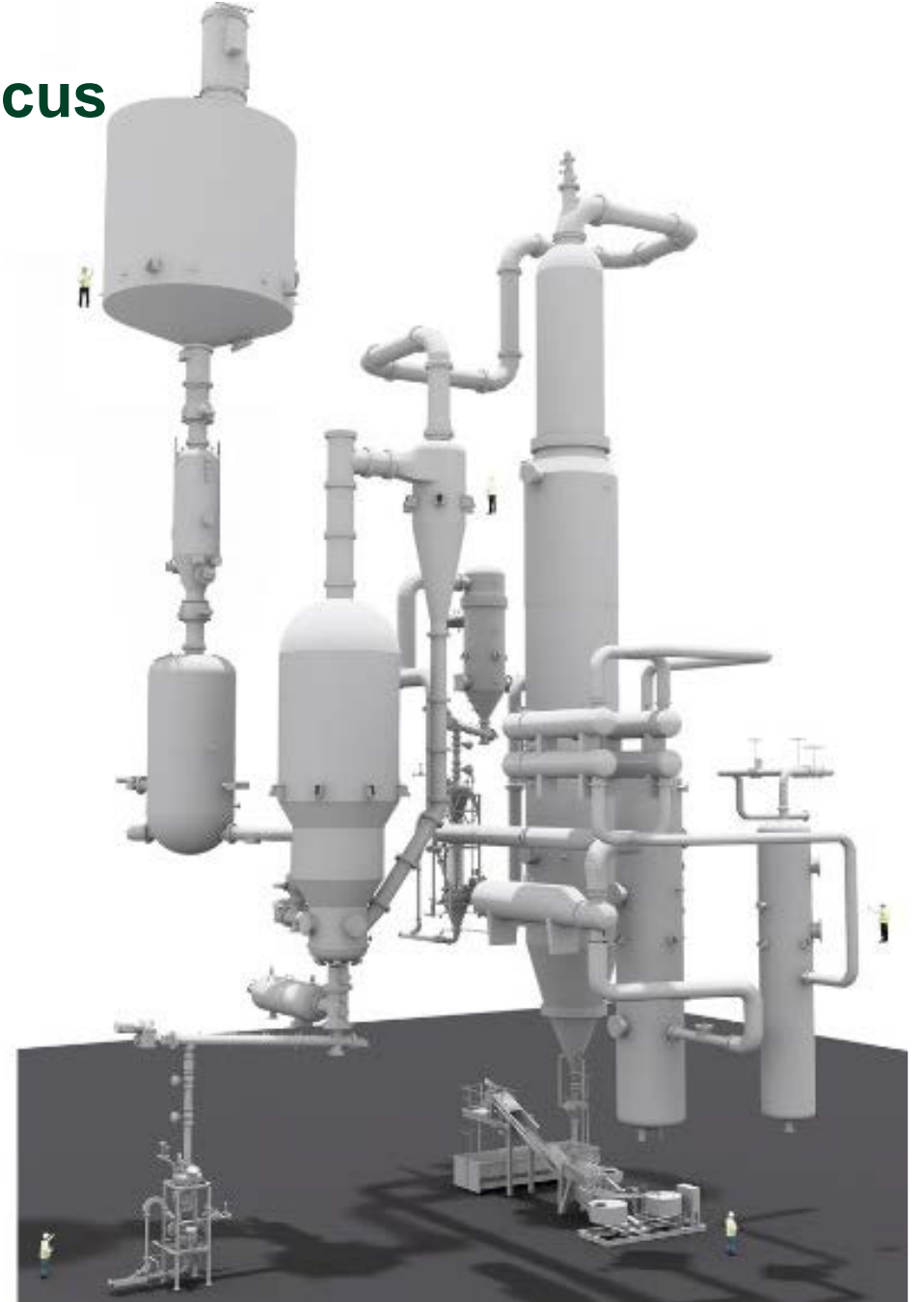
SunGas standardized S1000 gasification island 13
